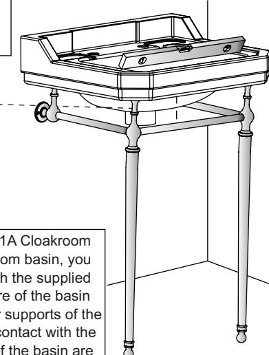
If you are installing the T21A Cloakroom basin stand with a cloakroom basin, you **MUST** install the basin with the supplied wall brackets. The structure of the basin does not allow for the rear supports of the basin stand to come into contact with the basin. The wall brackets of the basin are the supporting feature.
