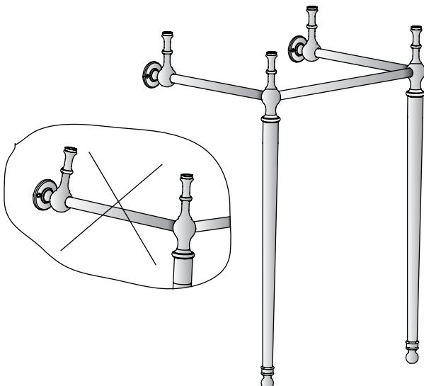
**5** Determine the final installation position and mark the 4 wall and two floor fixing hole positions in pencil.
