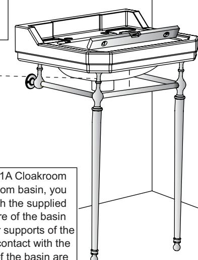
If you are installing the T21A Cloakroom basin stand with a cloakroom basin, you **MUST** install the basin with the supplied wall brackets. The structure of the basin does not allow for the rear supports of the basin stand to come into contact with the basin. The wall brackets of the basin are the supporting feature.
