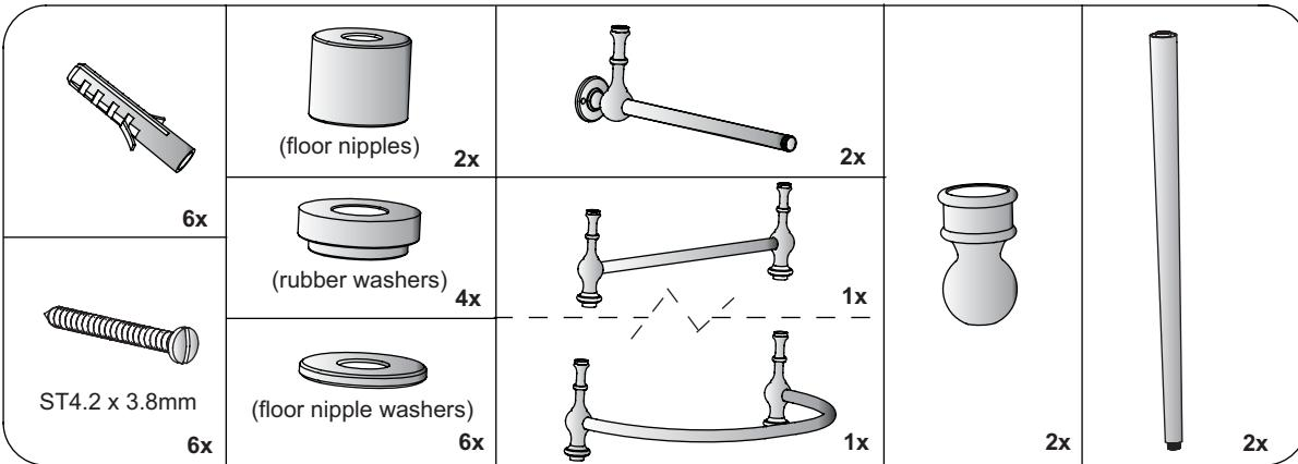
**1** Attach the two horizontal rails to the front rail.
