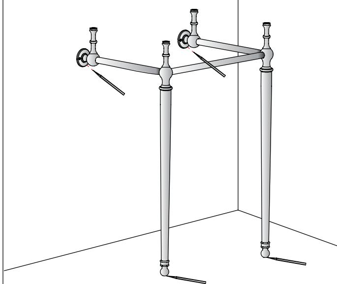
**6** Using a 6mm drill bit drill the six holes on the marked positions (note: In the event that the wall / floor fixings supplied being inappropriate for the wall / floor, please source alternatives).
