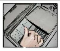
2. Open the fireplace cover and insert a narrow tool, e.g. a screw-driver, in one of the holes in the centre stone (always start with the centre stone).
